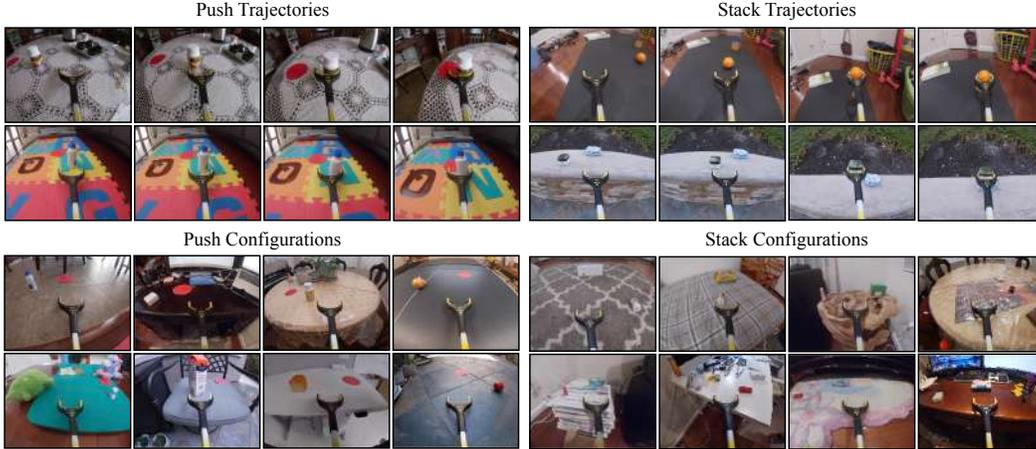
**Figure 3:** For both Pushing (left) and Stacking (right), we collect 1000 trajectories each with diverse objects and scenes. The top two rows depict 4 frames from single trajectories, while the bottom two rows depicts the variations in environments collected in our dataset.
